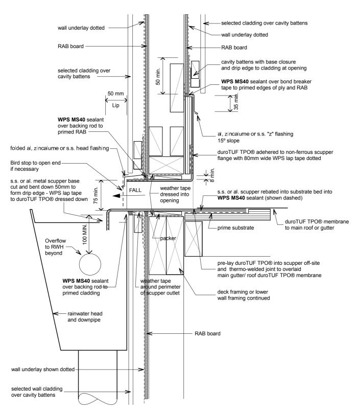
duroTPO-T05 - duroTUF TPO® Outlet Scupper Section
