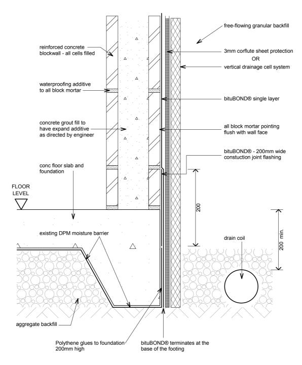
bitu-B23 - Blockwall Foundation type 2
