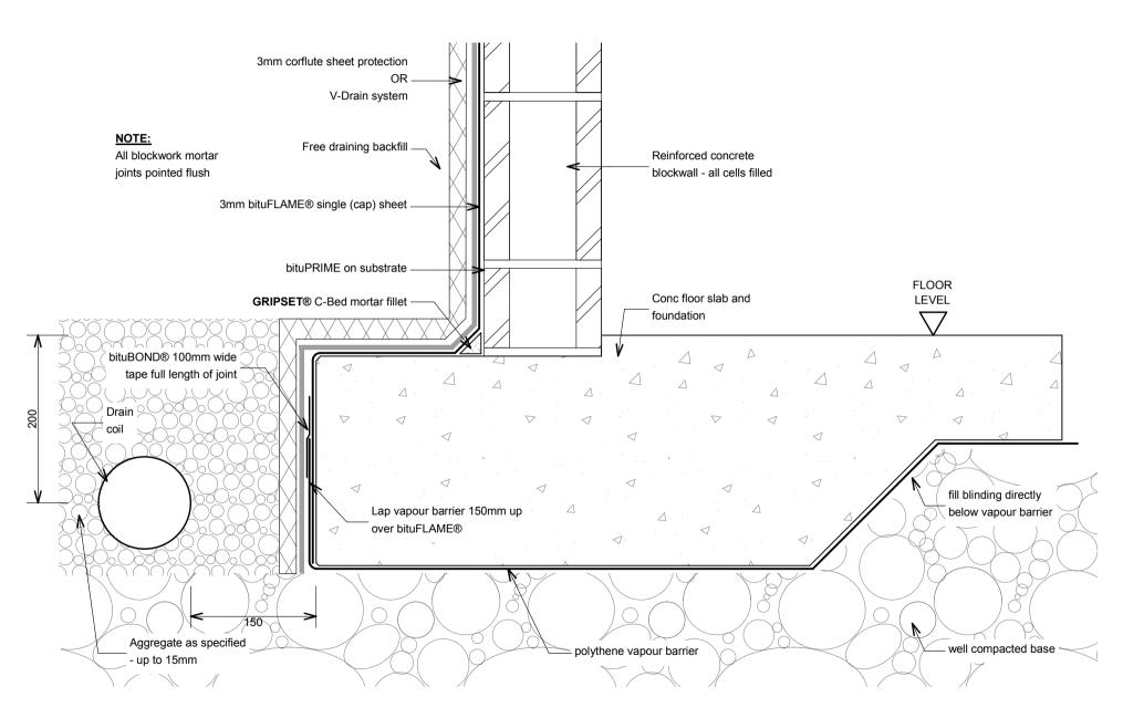
bF-T20 - Blockwall/ Floor Joint 1-1 (single layer)
