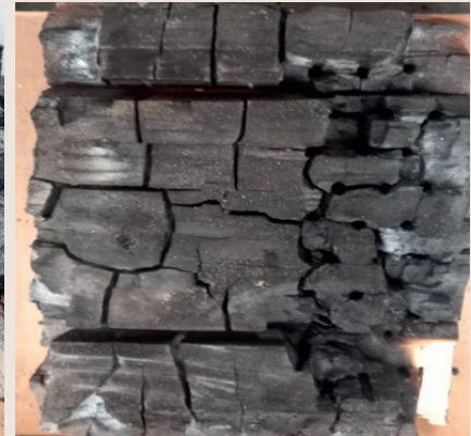
Figure 10. Increased charring below a metal plate (plan view showing screw holes on right hand side). (Credit: E. Claridge)
