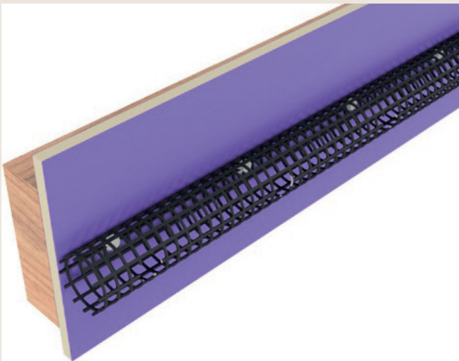
Figure 13. Intumescent cavity barrier – A fire rated intumescent mesh fixed onto rigid air barrier in a ventilated cavity at the level of a timber floor (Courtesy Ryanfire, 2023)
