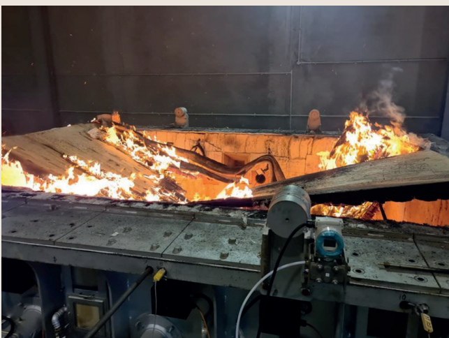
Figure 6. Structural collapse of a timber floor during testing, after failure criteria have been met (Credit: Fire TS Laboratory)
