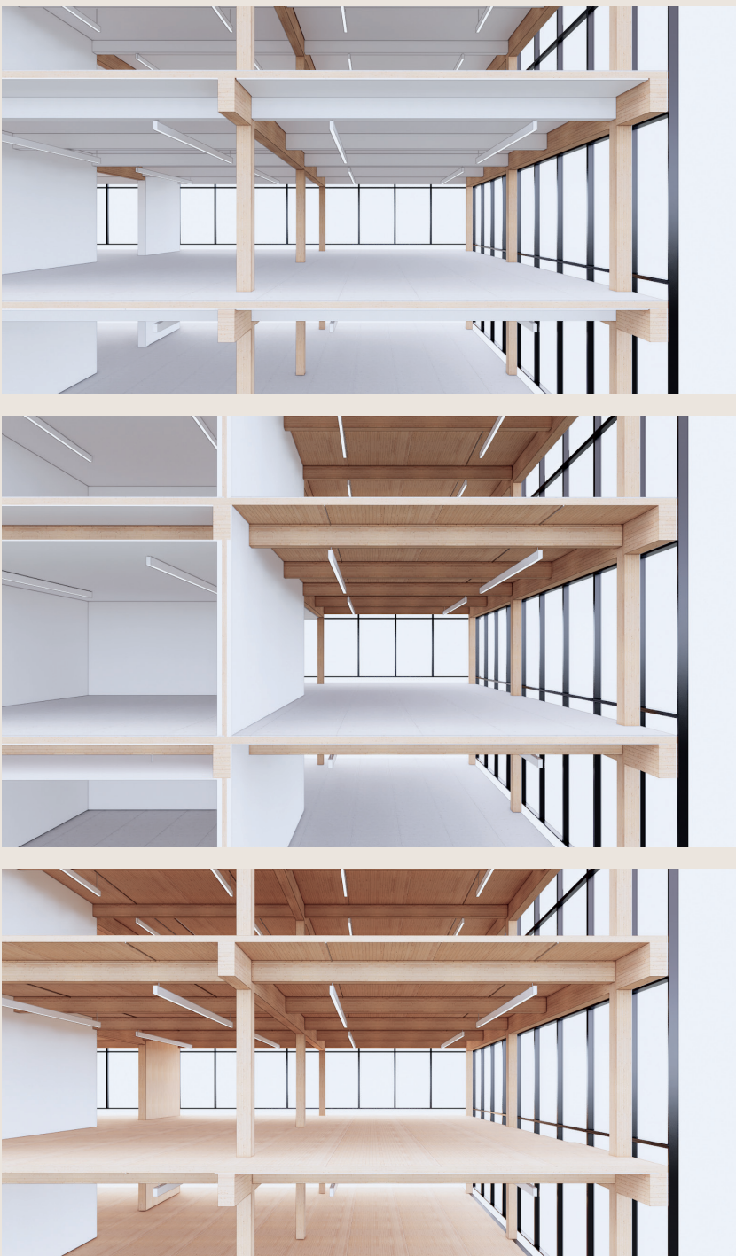
Figure 1. Decreasing levels of encapsulation, from top image to bottom image (Credit: Studio Gang Architects, San Francisco, USA)
