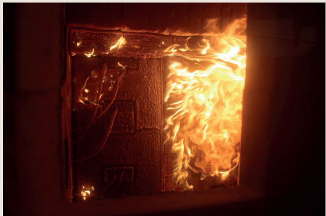
Figure 2. Inside the furnace of a CLT test, Intumescent coating (left) and non-encapsulated (right) (Credit: Fire TS Laboratory)
