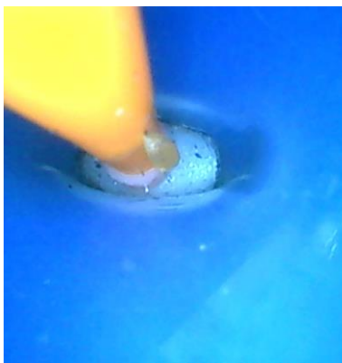
The PULL THRU™ Cleaning Brush in the kinked biopsy channel
