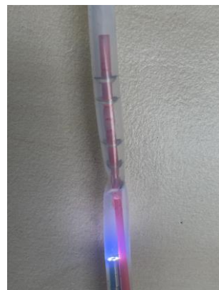
The PULL THRU™ Cleaning Brush in the kinked biopsy channel, outside the endoscope
