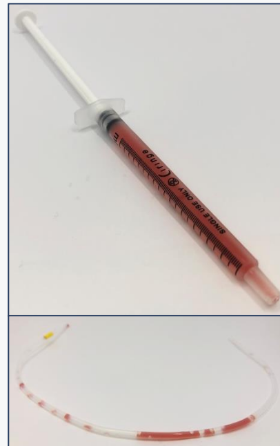
Figure 2. 1mL Syringe of diluted test soil and inoculated PTFE tubing
