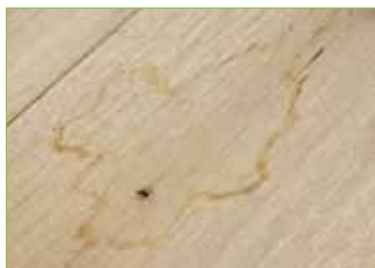
Ugly water marks can quickly appear due to insufficient resistance against liquids.
