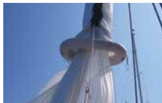
**3.** Snuffair is hoisted and dropped using the up/down line within the rope pocket.
