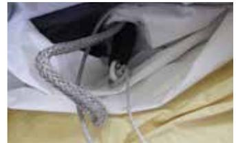
**3.** To connect the head strop to the spinnaker put head-strop loop through head of spinnaker and replace dog-bone. Lash securely in place.
