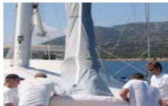
**3.** Sock the spinnaker for the first time by hoisting with the bucket at the top of the spinnaker then pulling the bucket down over the sock during the hoist process
