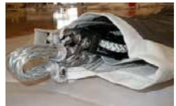
**6.** The spinnaker halyard can now be attached to the other end of the head strop. **For rope pocket socks:** Make sure down-line feeds correctly around block on headstrop
