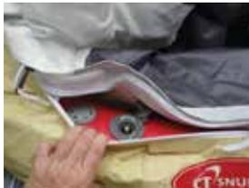
**1.** Inflation/pressure relief valves are accessed through the lower zip on the chafe guard. *The relief valve releases air at 10PSI.*
