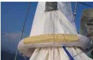
**2.** Sock the spinnaker for the first time by hoisting with the bucket at the top of the spinnaker then pulling the bucket down over the sock during the hoist process.
