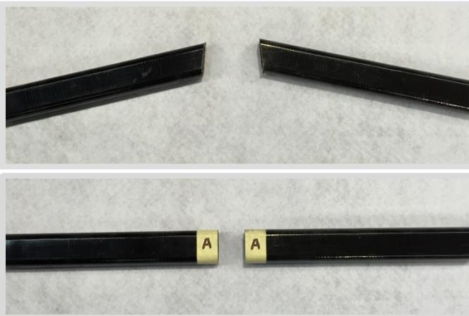
2. Ensure that the internal surface of the batten sections are **sanded in preparation for bonding.**
