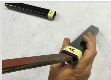
3. Dry fit the internal joiner to each section before bonding.
