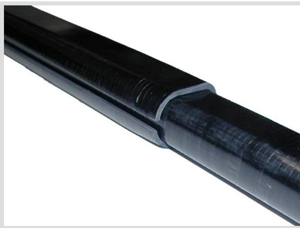
7. Cut the carbon sock to lengths slide over the repair and laminate into position with epoxy resin. Leave to cure.
